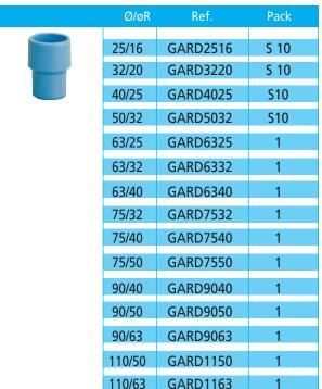
NB: reducer's large ends for references GARD 32 to 110 (except GARD 7532, 7540 and 7550) can be used as sockets and spigots, with one size interval. Small ends are socket only. e. g.: GARD 90/63 = 90 SPIG. + 75 SOC. / 63 SOC.
